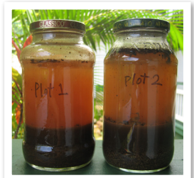
After settling for at least 24 hours, organic matter has formed a distinct layer at the very top inside the jars.
